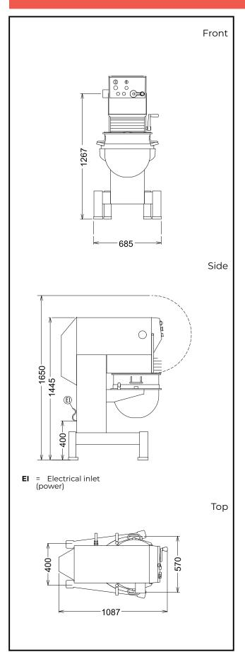
Electric 220-240/380-415 V/3 ph/50 Supply voltage: Electrical power, max: 1.54 kW **Total Watts:** 1.54 kW Capacity: ISO 9001; ISO 14001 kg/ Performance (up to): Cycle Capacity: 60 litres Key Information: External dimensions, 685 mm Width: External dimensions, 1087 mm Depth: External dimensions, Height: 1445 mm **Shipping weight:** 337 kg ISO 9001; ISO 14001 kg with Spiral hook
